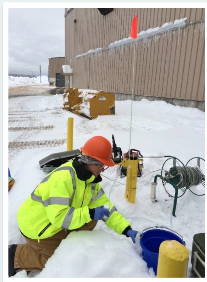
CEMP Field Technician Abbie Debiak sampling well QALo29A at the Eagle Mine for the Ground Water Discharge Permit Monitoring
