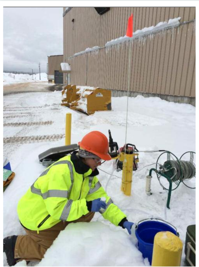
CEMP Field Technician Abby Debiak sampling well QAL029A at the Eagle Mine for the Ground Water Discharge Permit.
