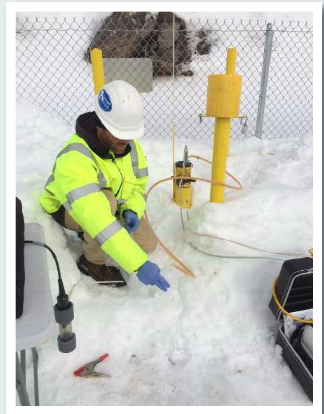
CEMP Field Technician, Hunter King, collecting a groundwater sample at the Humboldt Mill
