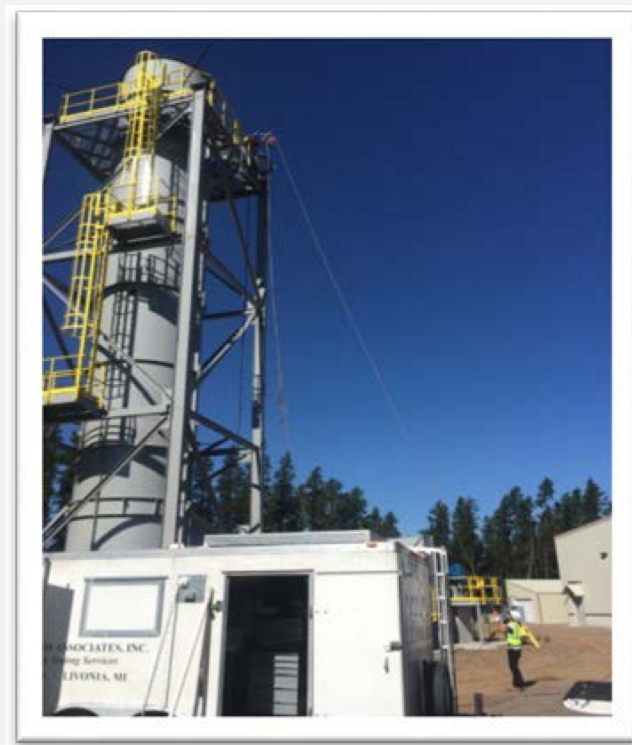
The CEMP deployed the portable air monitoring equipment to collect ambient air quality data at the Mine Ventilation Air Raise (MVAR) during the Michigan DEQ required stack test on September 16.
