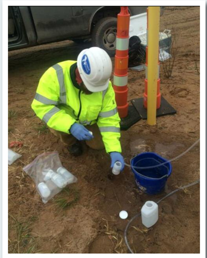
CEMP Field Technician conducting Groundwater Discharge Permit Sampling.
