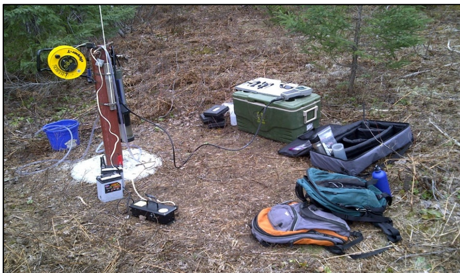
Monitoring well sampling set-up
