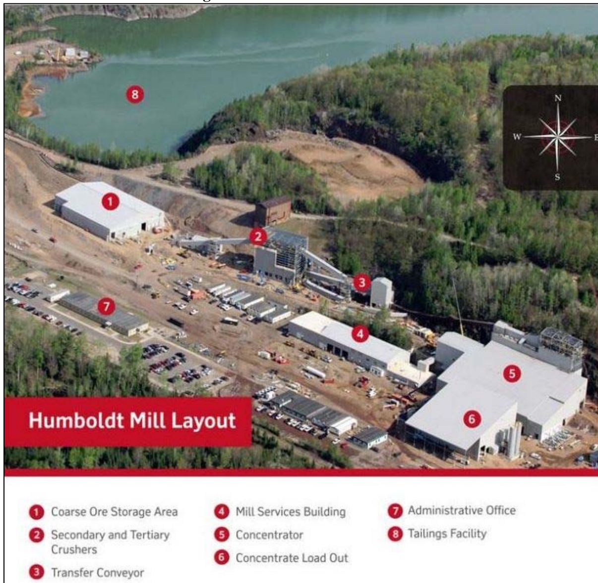
Diagram of Humboldt Mill Facilities
