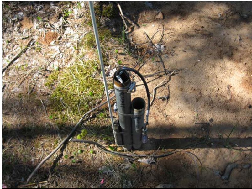
Piezometer with a level troll located over the ore body; QAL043A.
