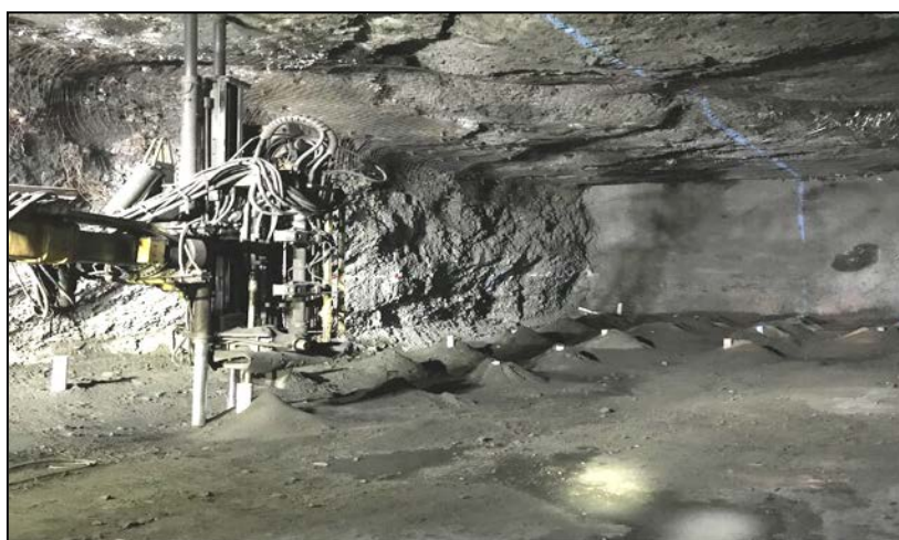
Longhole drill, drilling a production stope in Eagle
