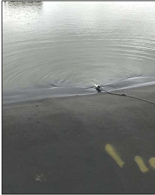
LLSI conducting the leak location survey on CWB #2 with a probe.
