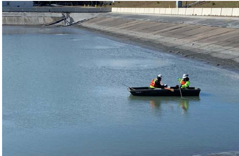
Sediment thickness test being performed on the basins, May 2020
